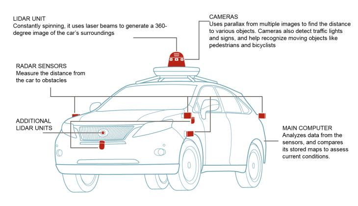
Figure 2: How an Autonomous Vehicle Drives Itself
