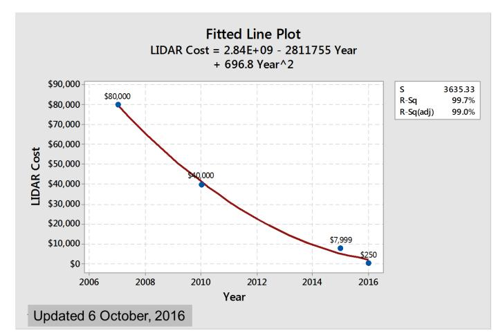
Figure 8: Autonomous Vehicle Technology Cost is Decreasing Exponentially – LIDAR Example
